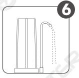
**Step 6:**Let the water run through the filter for 5 minutes to rinse out the new cartridae.
